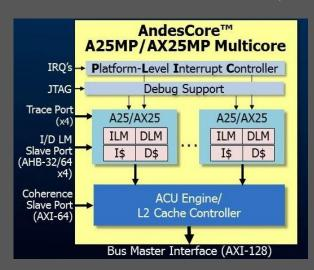
generation 32-bit A25MP and 64-bit AX25MP RISC-V Multicore Processors with Andes Custom Extensions, that allows designers to create special instructions to accelerate compute intensive functions, a capability highly desired in AI and ADAS designs. The cache coherent A25MP and AX25MP RISC-V multicore processors are the company's first with comprehensive DSP instruction extension based on the RISC-V P-extension draft Andes donated to the RISC-V Foundation.
