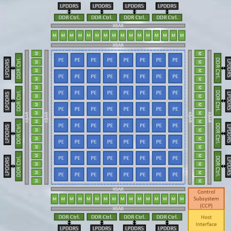
Figure 3: High-level architecture of the accelerator
